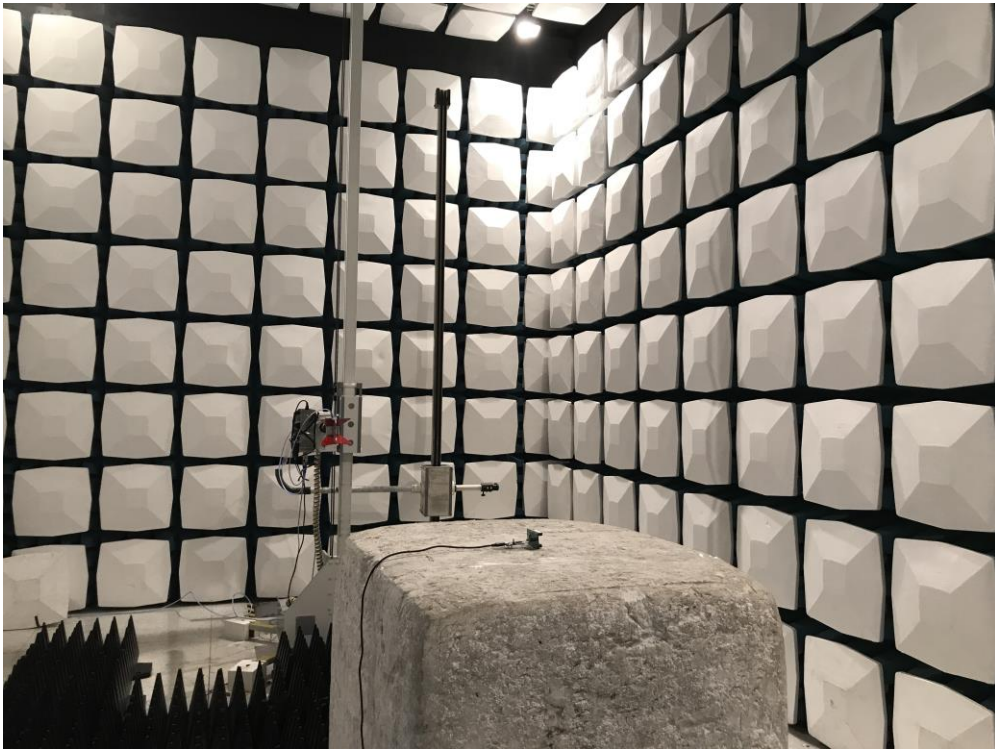
Description: Radiated Emission Test Setup for 1~18GHz
