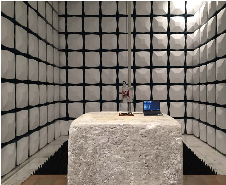
Description: Radiated Emission Test Setup for 1~18GHz
