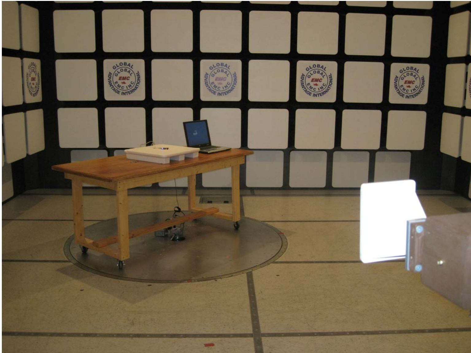
Figure 1 – EUT Radiated emission setup 1
