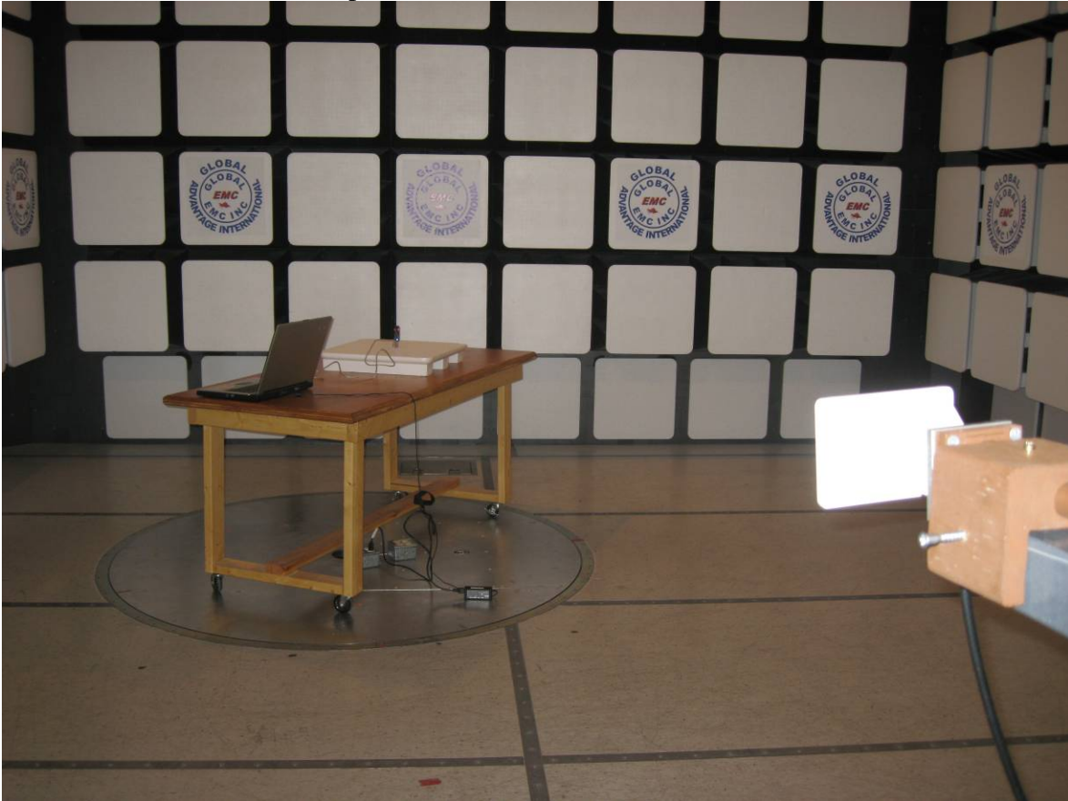
Radiated Emissions Test Setup Photo 2
