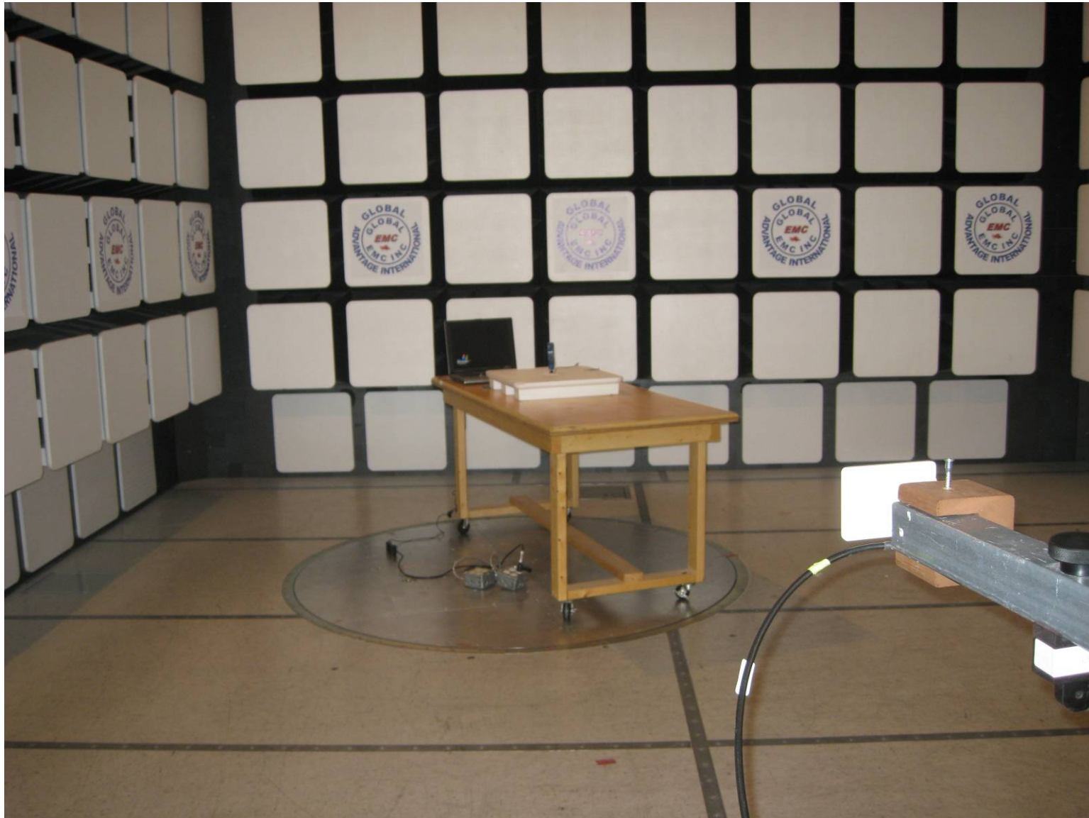
Figure 1 – EUT Radiated emission setup 1
