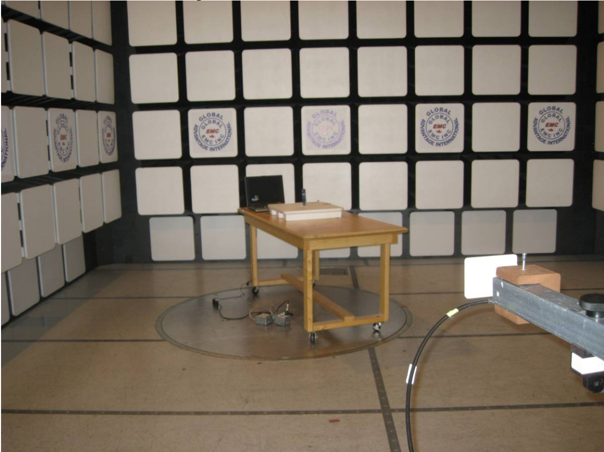
Radiated Emissions Test Setup Photo 1
