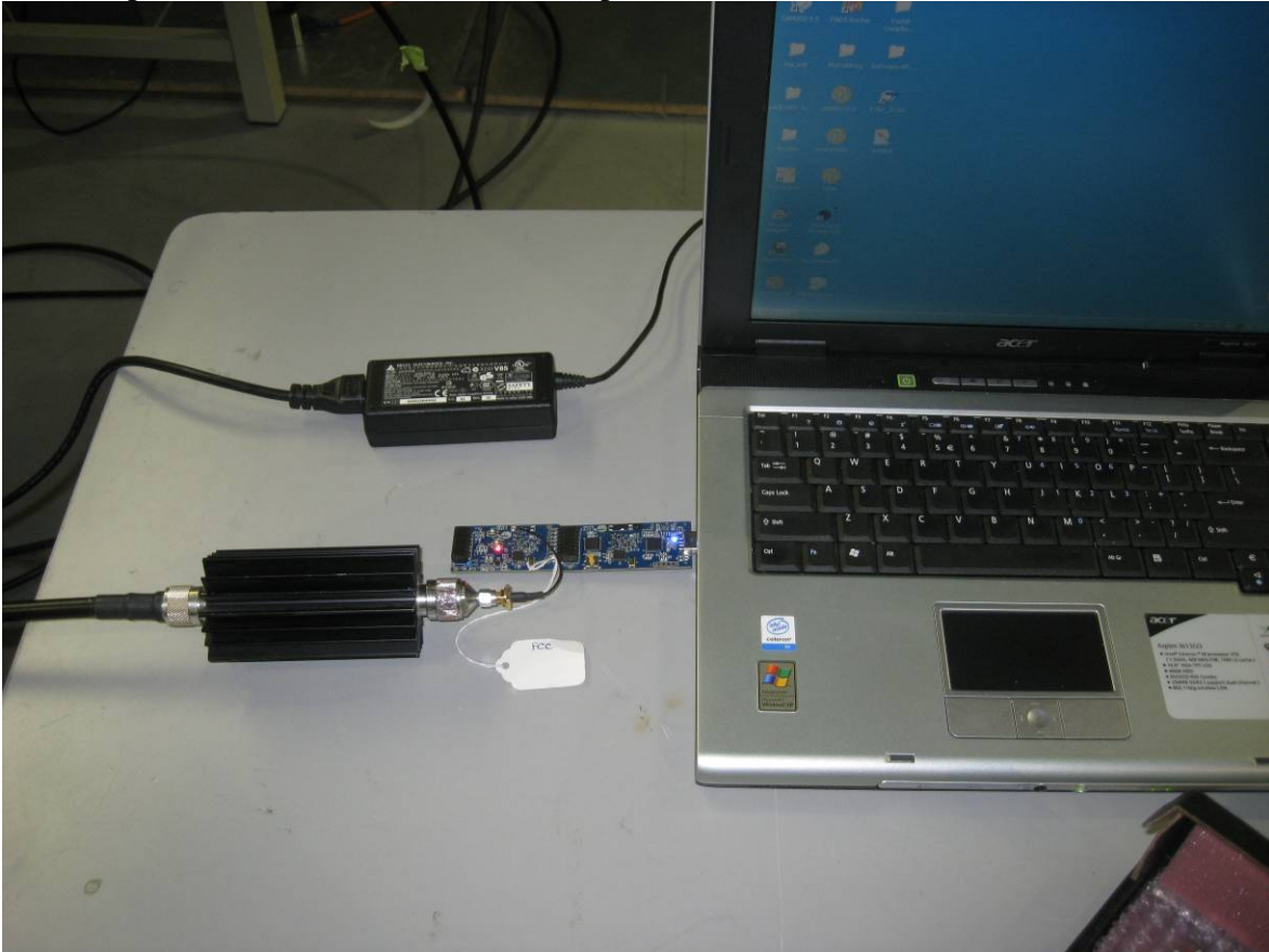
Antenna port conducted emissions test setup
