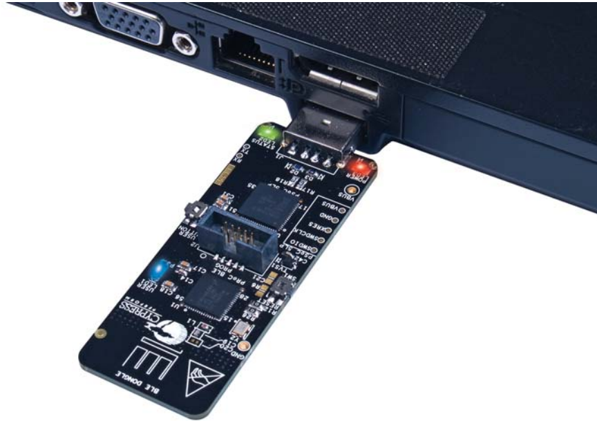
Figure 6-60. Connect Dongle to USB Port
