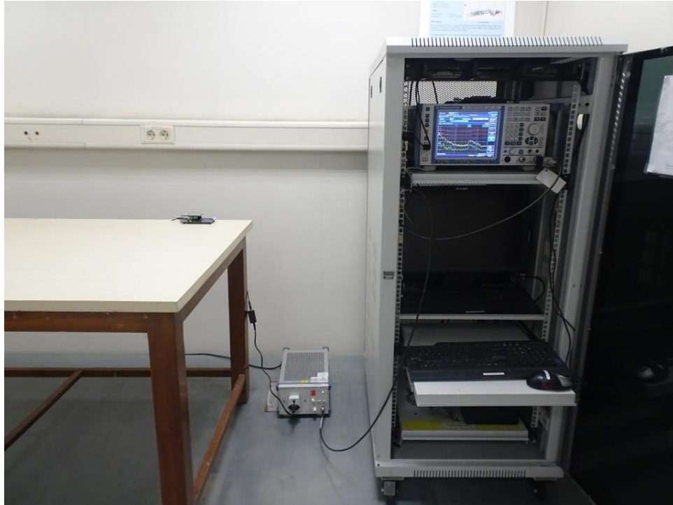
Test setup: AC power line conducted emission test
