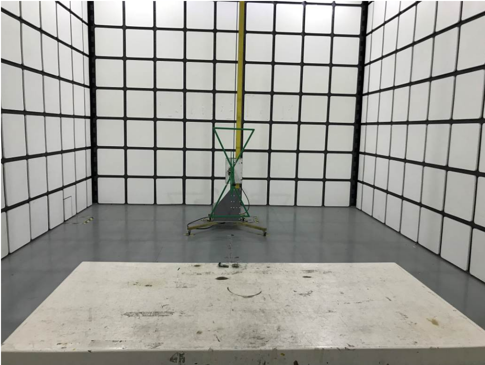
Description: Radiated Emission Test Setup for 1~18GHz
