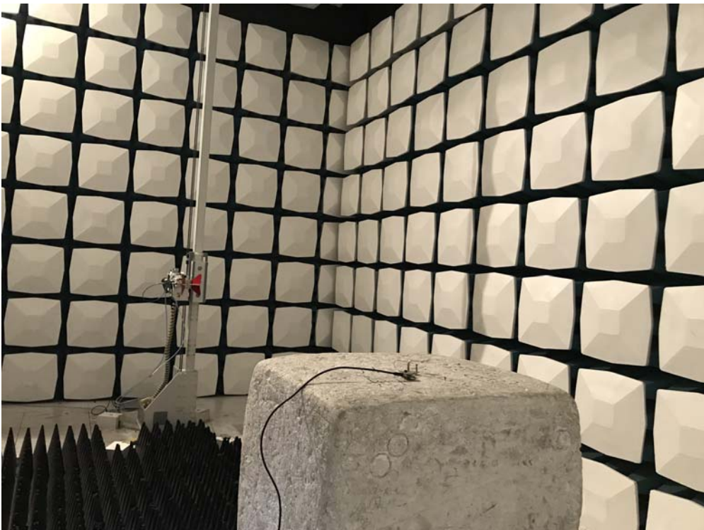
Description: Radiated Emission Test Setup for 1~18GHz
