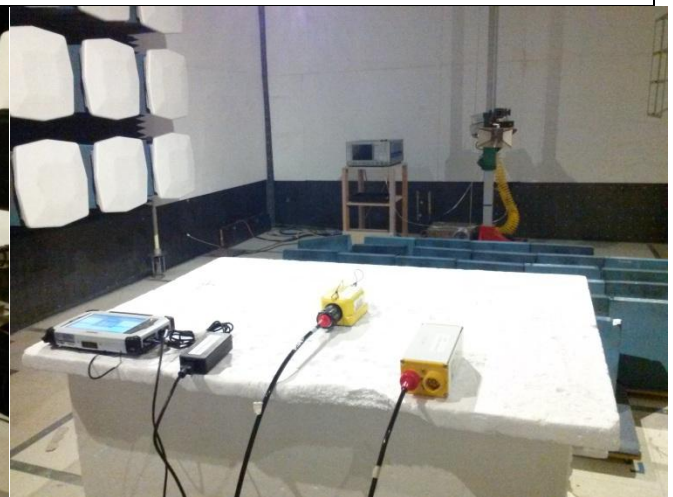
Radiated Emissions (>1GHz) – Rear View
