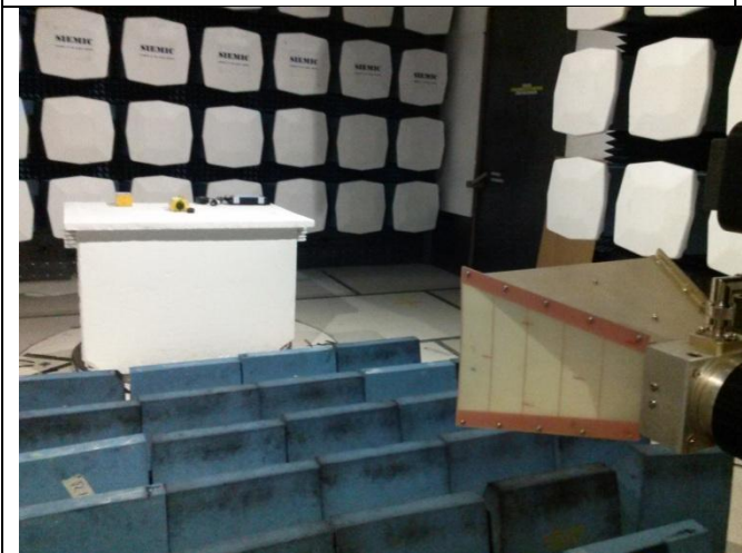
Radiated Emissions (>1GHz) – Front View
