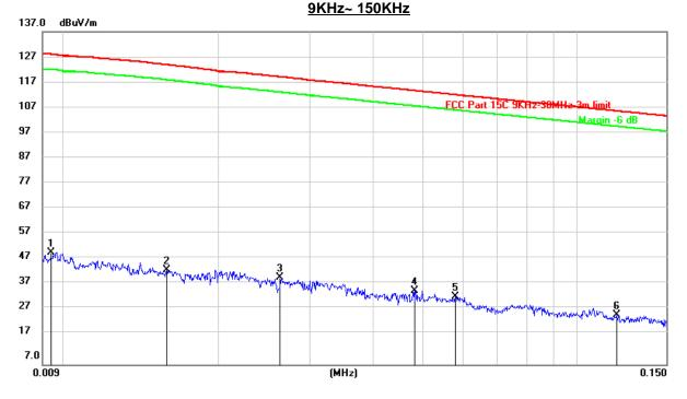
Reading Correct Limit No. Frequency Result Margin Remark (dBuV/m) (MHz) (dBuV/m) dB/m (dBuV/m) (dB) 20.26 -77.31 1 0.0094 30.49 50.75 128.06 peak 2 20.27 43.83 124.11 0.0158 23.56 -80.28 peak 20.75 20.31 41.06 -78.30 3 0.0263 119.36 peak 4 20.31 35.71 113.95 -78.24 0.0483 15.40 peak 5 -78.86 0.0580 13.19 20.31 33.50 112.36 peak 0.1198 6.03 20.30 26.33 106.04 -79.71 6 peak
