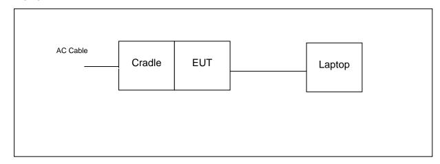
Note: The cradle can transform AC 120V to DC 12V and the EUT can be charged by the cradle.
