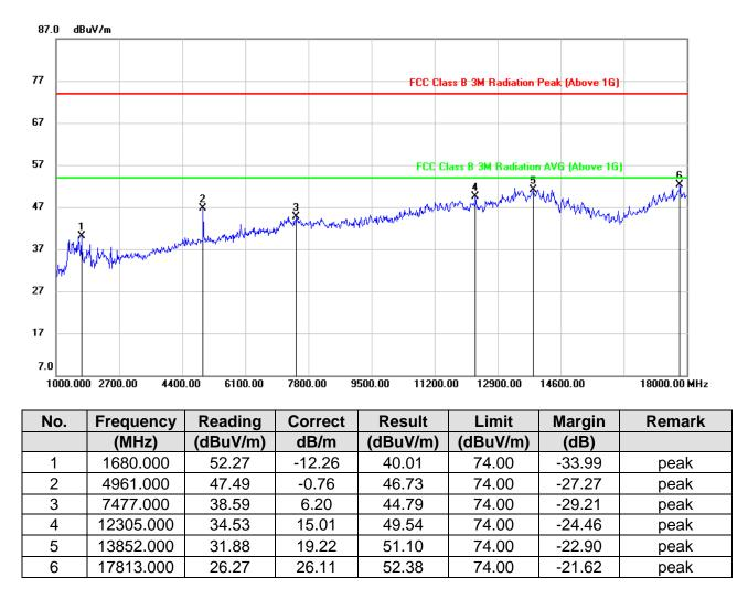
Note: 1. Measurement = Reading Level + Correct Factor.
