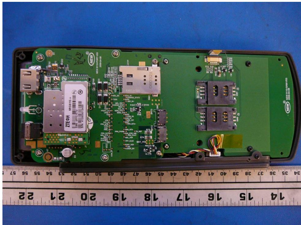
**EUT - RF Module with Shield on Front View**
