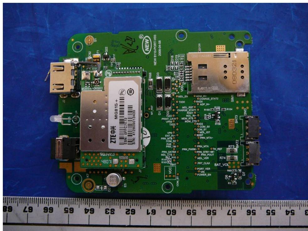
**EUT - RF Module Back View**
