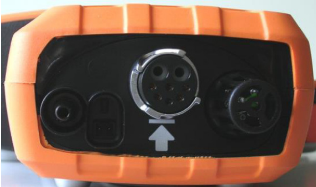
t330i, connections for AC/DC adapter and flue gas probe, temperature sensor
