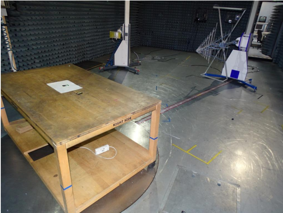
Photo 1: Test setup for radiated measurements (stand-alone, EUT supplied by a battery, unintentional radiator §15.109, ANSI C63.4) 30 MHz – 1 GHz
