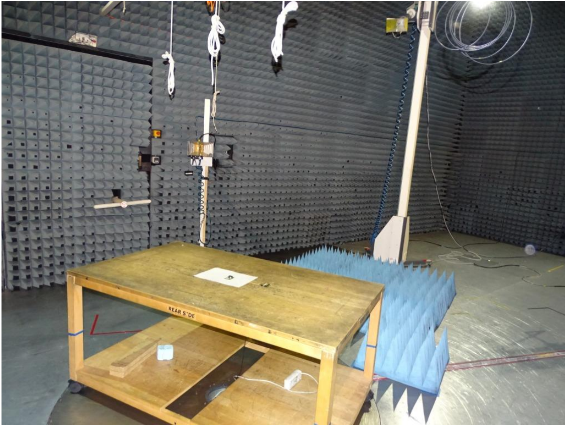
Photo 2: Test setup for radiated measurements (stand alone, EUT supplied by a battery, unintentional radiator §15.109, ANSI C63.4) Above 1 GHz
