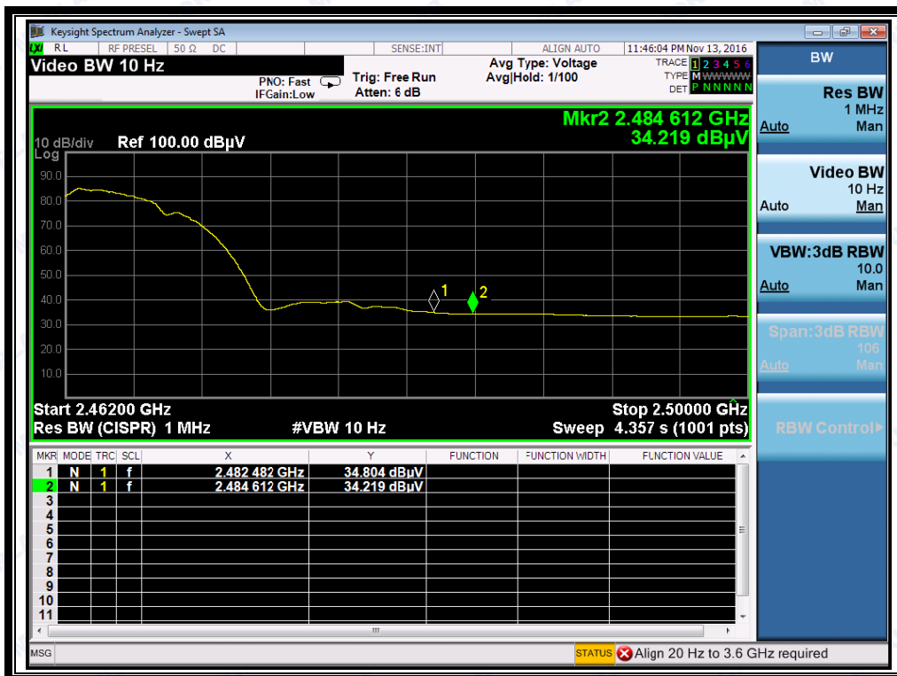
(Plot B2: Channel = 11 AVG @ 802.11b)
