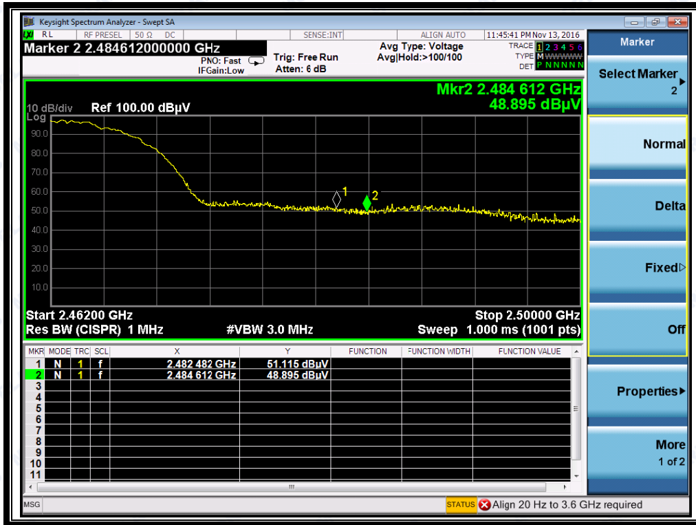
(Plot B1: Channel = 11 PEAK @ 802.11b)
