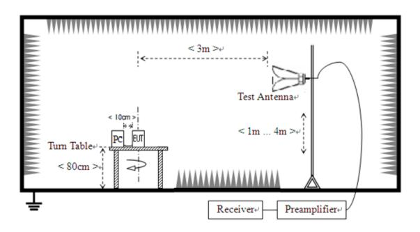
The test is performed in a 3m Semi-Anechoic Chamber; the antenna factor, cable loss and so on of
