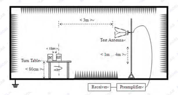
The test is performed in a 3m Semi-Anechoic Chamber; the antenna factor, cable loss and so on of
