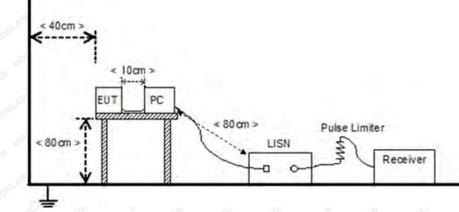
The EUT is placed on a 0.8m high insulating table, which stands on the grounded conducting floor, and keeps 0.4m away from the grounded conducting wall. The EUT is connected to the power mains through a LISN which provides  $50\Omega/50\mu$ H of coupling impedance for the measuring instrument. A Pulse Limiter is used to protect the measuring instrument. The factors of the whole test system are calibrated to correct the reading.
