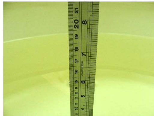
Fig 7.2 Photo of Liquid Height for Body SAR
