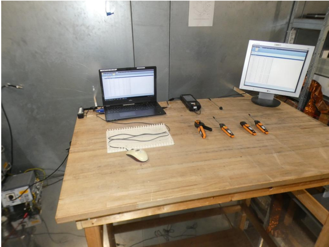
Photo 6: Test setup for conducted measurements (computer peripheral setup, EUT connected via USB-cable to computer, unintentional radiator §15.107, ANSI C63.4)
