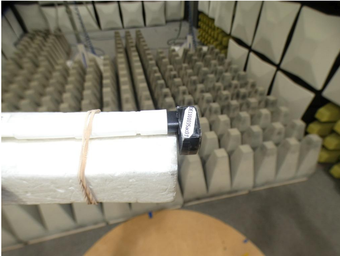
Photo 9: Test setup for radiated measurements, detailed view (stand alone, 1 – 18 GHz; FCC 15c247, ANSI C63.10)
