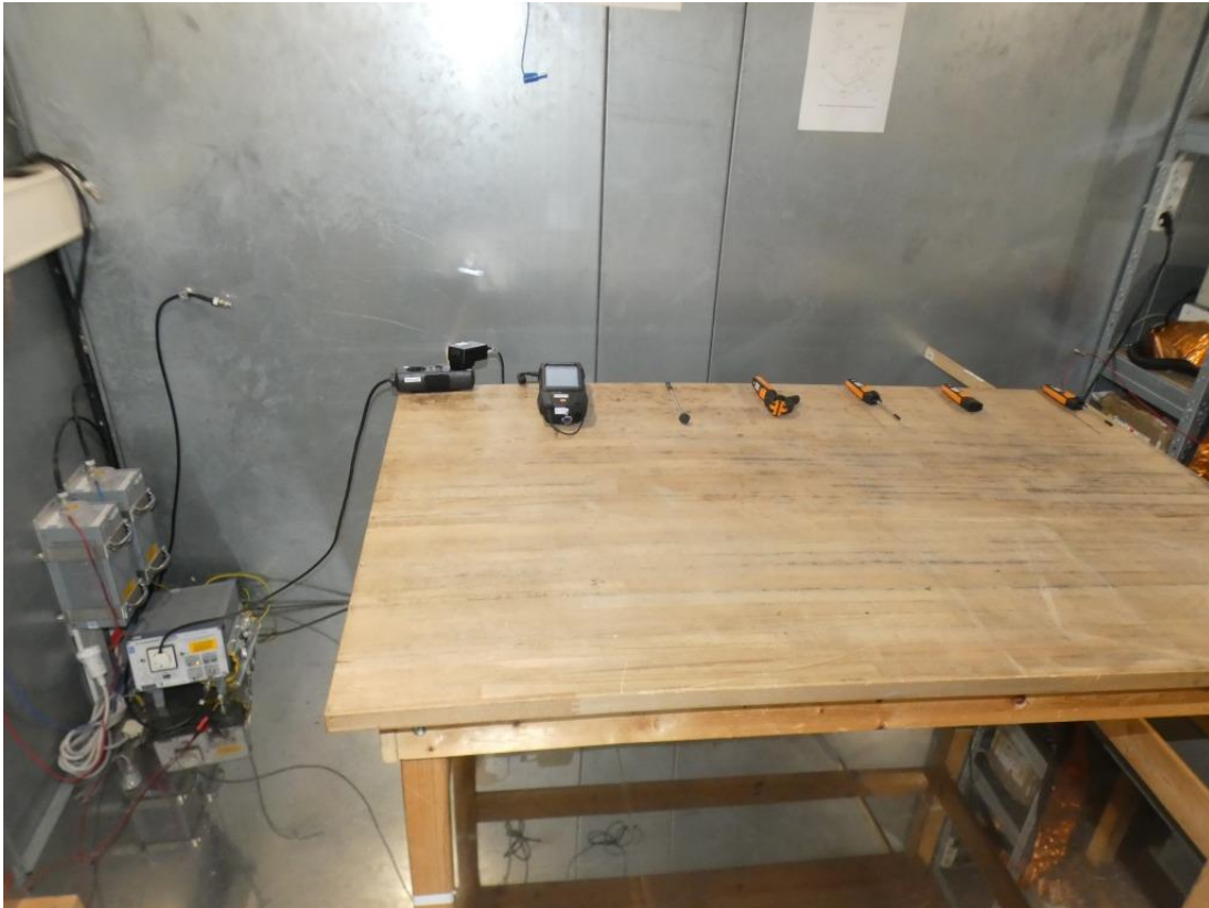
Photo 5: Test setup for conducted measurements (AC Port (power line), EUT supplied by AC/DC adapter, unintentional radiator §15.107, ANSI C63.4)
