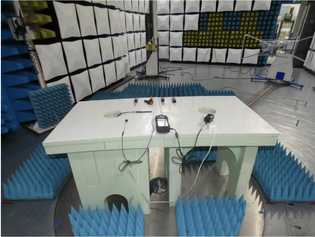
Photo 3: Test setup for radiated measurements (stand alone, semi-anechoic chamber above 1 GHz; unintentional radiator §15.109, ANSI C63.4)
