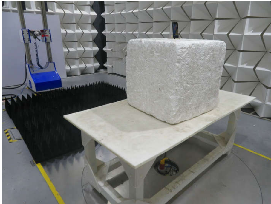
Radiated spurious emission Test Setup-3(Above 1GHz)
