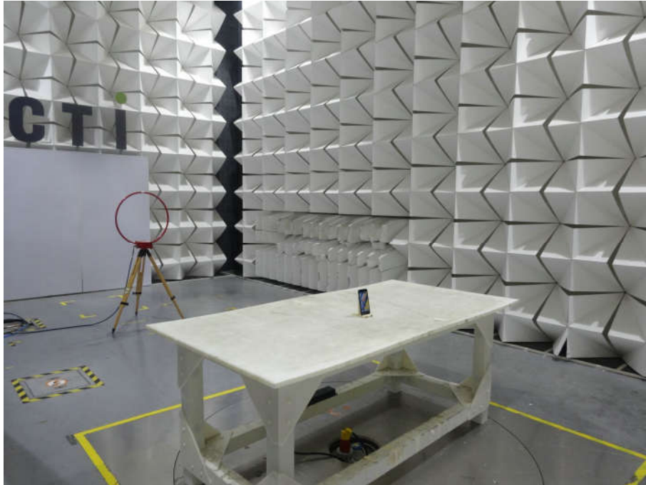
Radiated spurious emission Test Setup-1(9K-30M)
