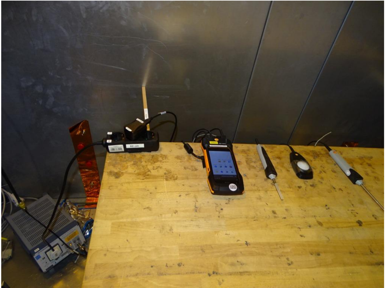
Photo 2: Test setup for conducted measurements (Test Setup:stand-alone, AC mains connection: connected via AC/DC Adapter, unintentional radiator §15.107, ANSI C63.4)
