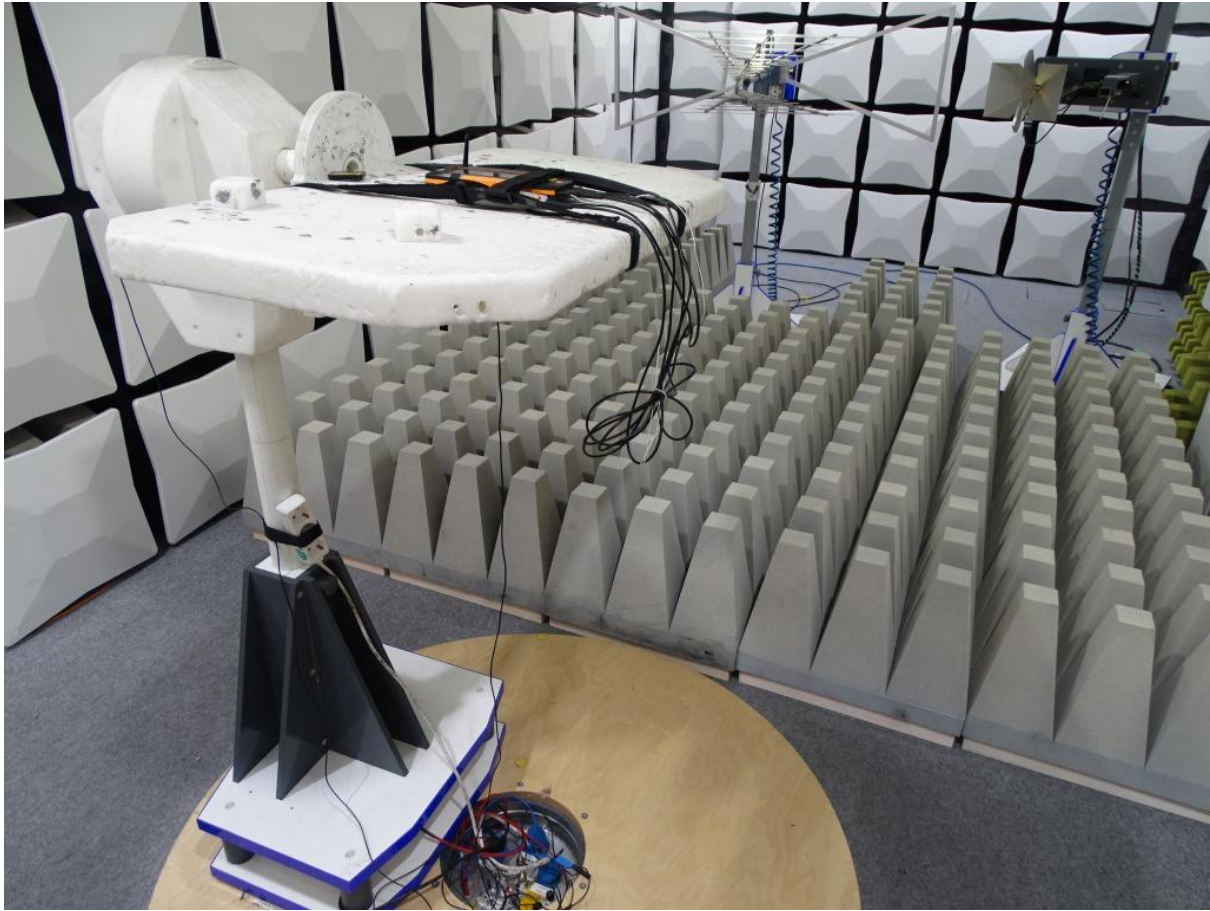
Photo 7: Test setup for radiated measurements (stand alone setup, 1 GHz – 24 GHz; FCC 15c247)
