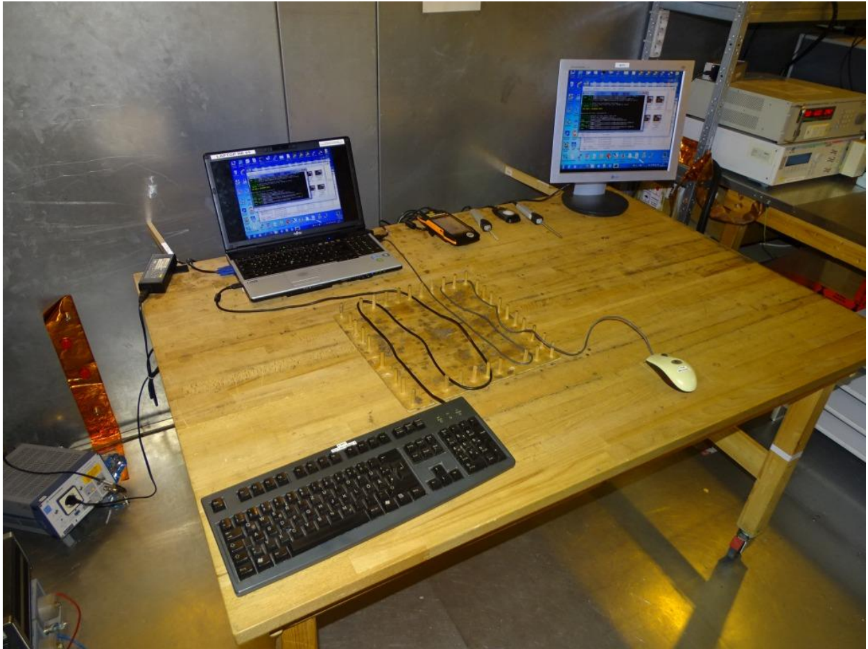
Photo 1: Test setup for conducted measurements (Test Setup:computer peripheral setup, AC mains connection: connected via computer device, unintentional radiator §15.107, ANSI C63.4)
