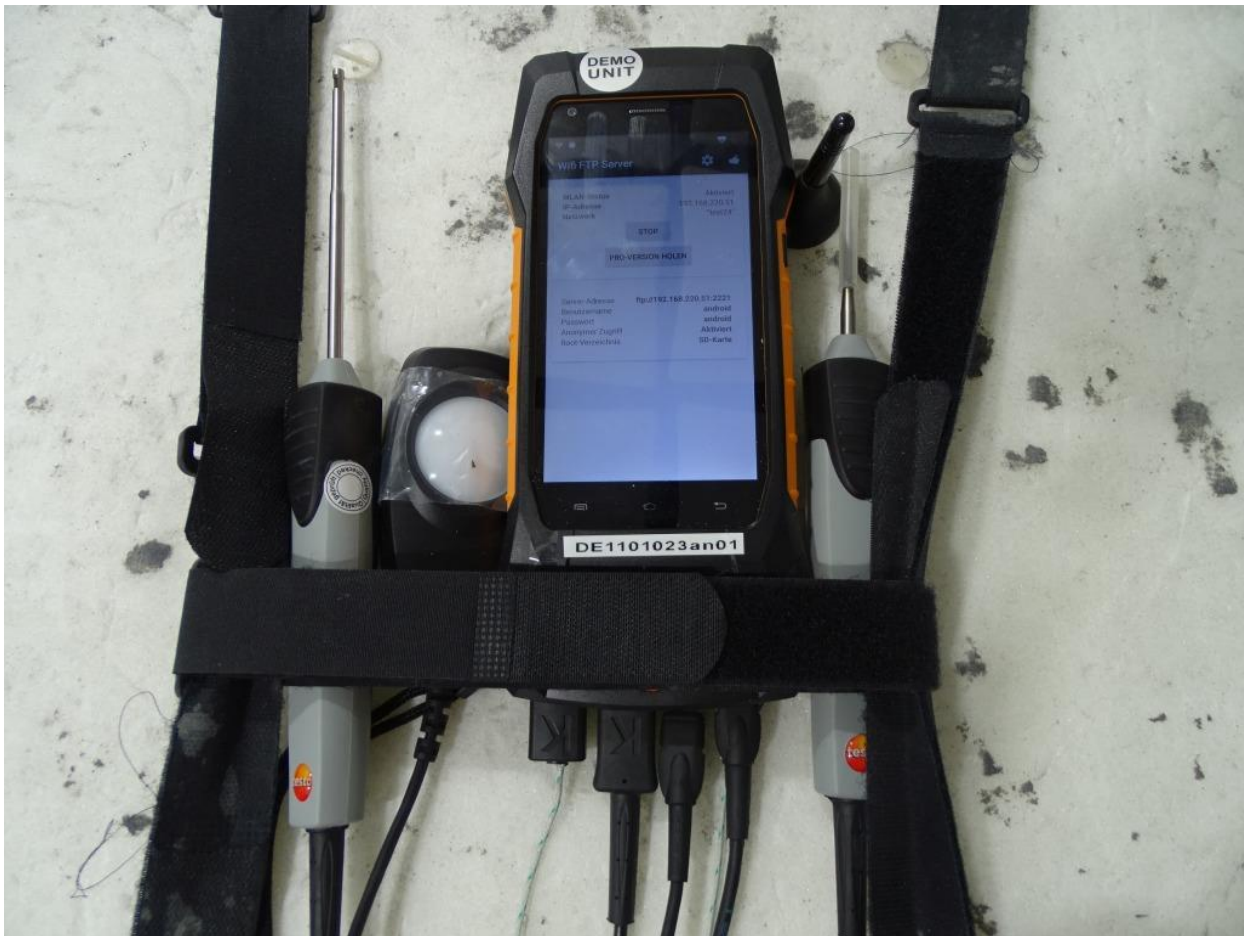
Photo 8: Test setup for radiated measurements, detailed view (stand alone setup, 1 GHz – 24 GHz; FCC 15c247)
