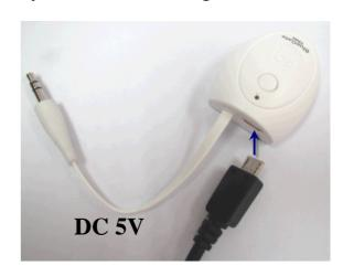
When the red LED is on, it is charging. When the red LED is off, it has charged full.
