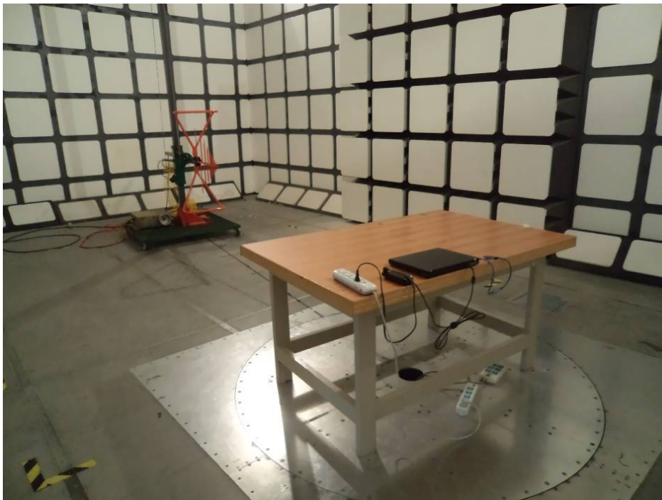
Below 1 GHz: Radiated Emissions - Rear View
