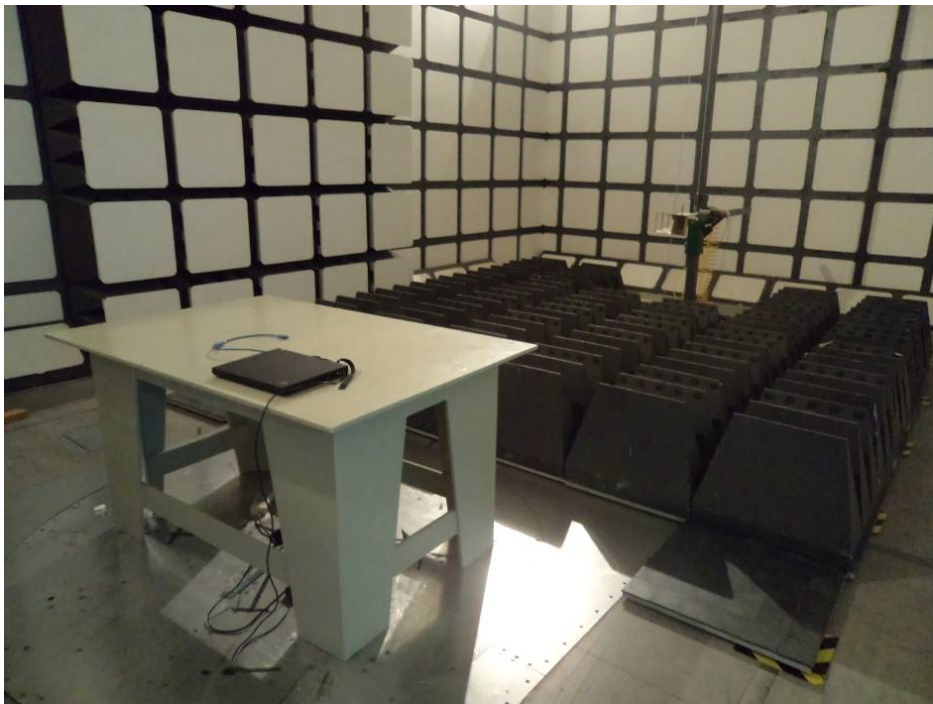
Above 1 GHz: Radiated Emissions - Rear View
