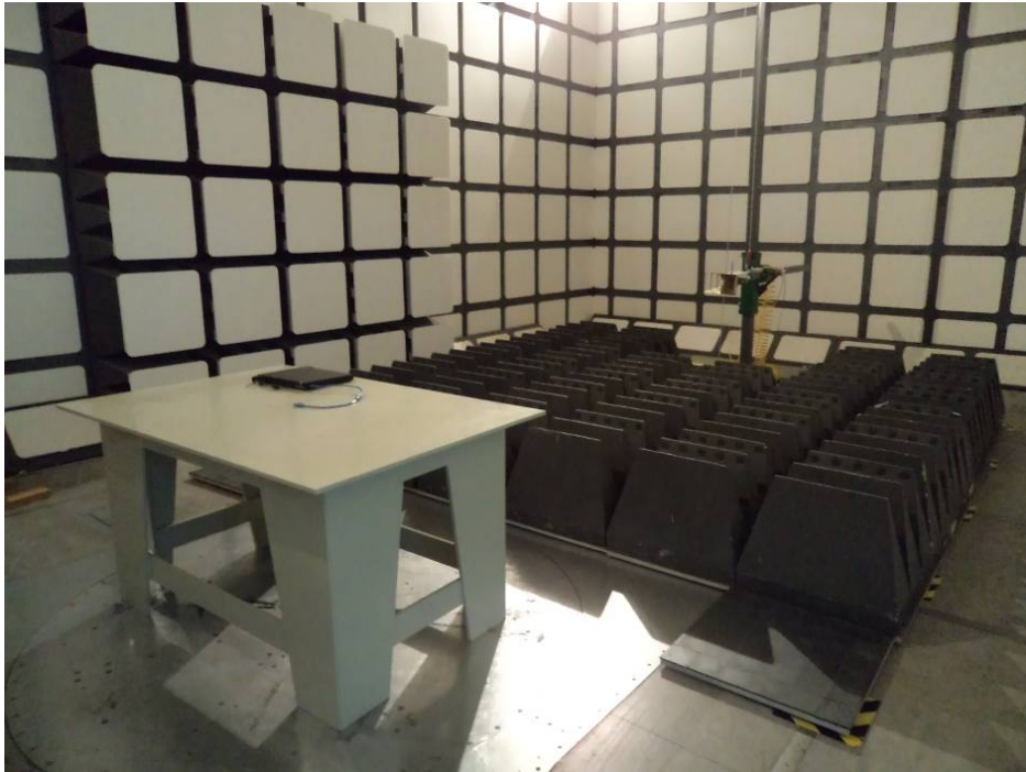
Above 1 GHz: Radiated Emissions - Rear View
