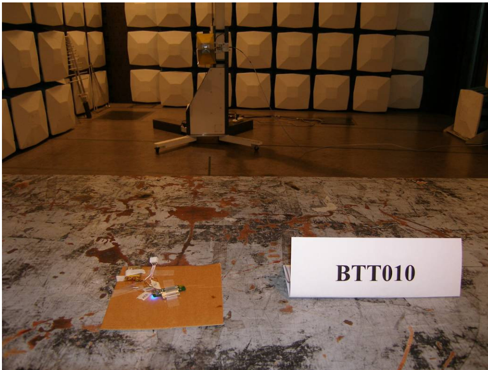
Photograph 2: Set-up for Radiation Measurement above 1GHz
