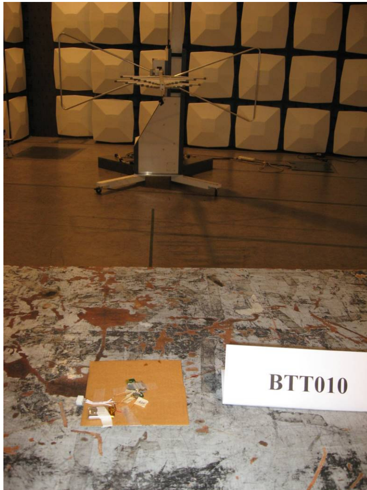
Photograph 1: Set-up for Radiation Measurement below 1GHz
