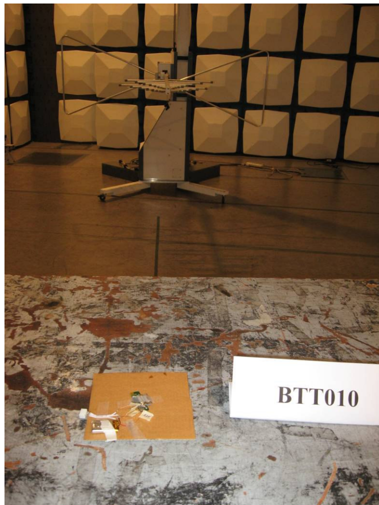
Photograph 1: Set-up for Radiation Measurement below 1GHz
