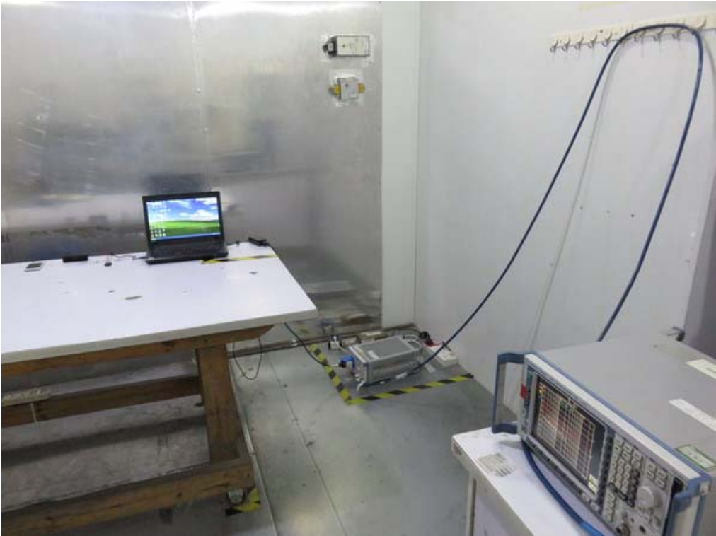
FCC RADIATED EMISSION TEST SETUP
