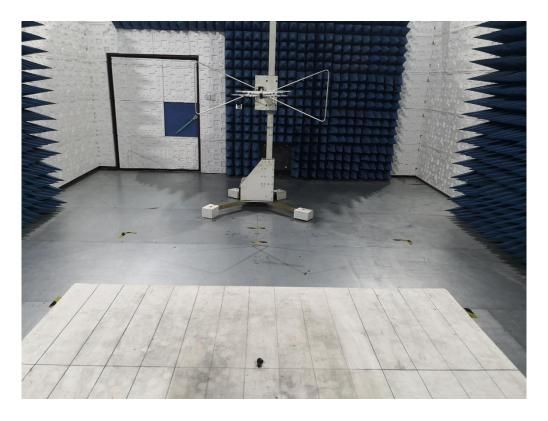
RADIATED EMISSION TEST SETUP ABOVE 1GHZ
