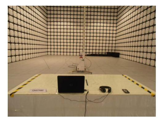
2 Set-up for conducted emission test
