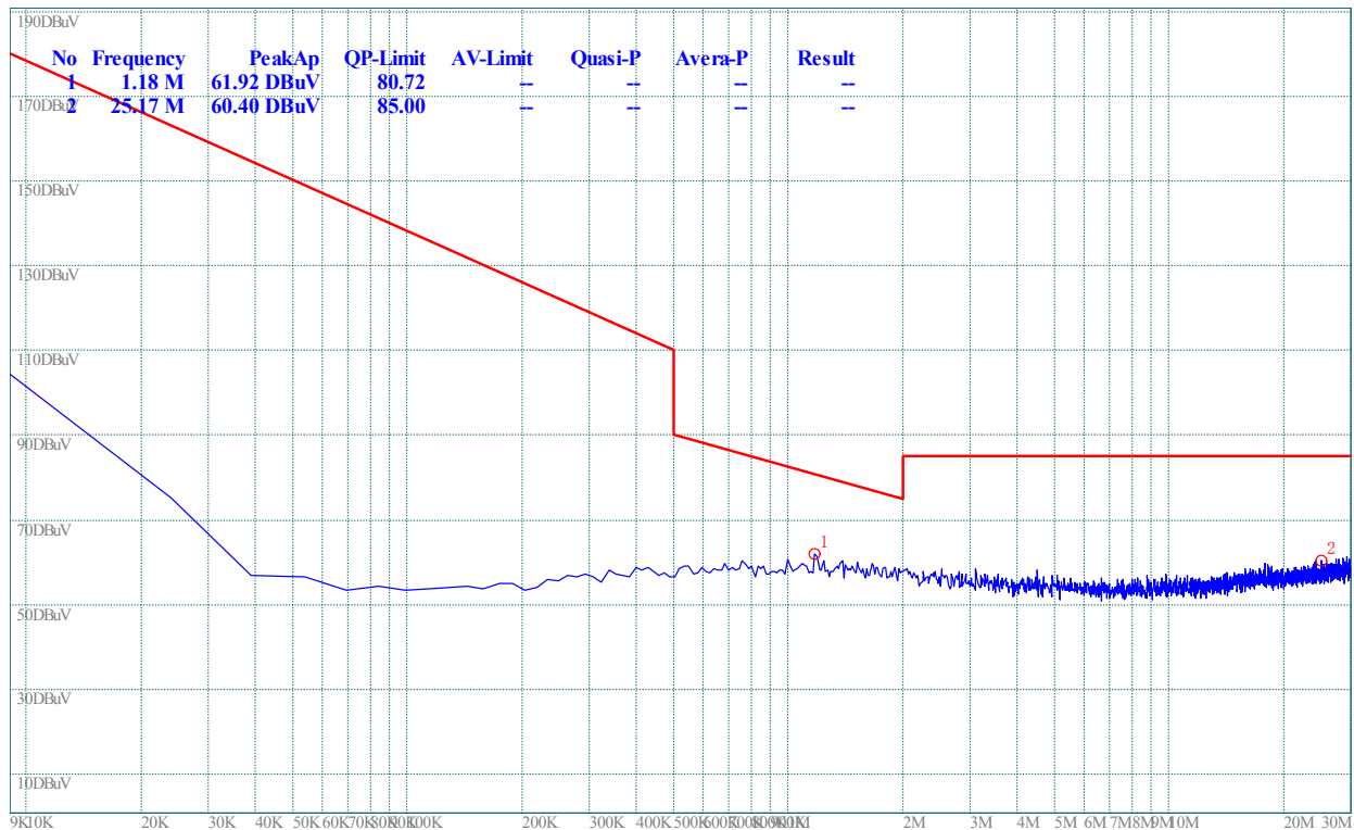
(Plot A.0: 9kHz to 30MHz @ 8-DPSK, channel 0)
