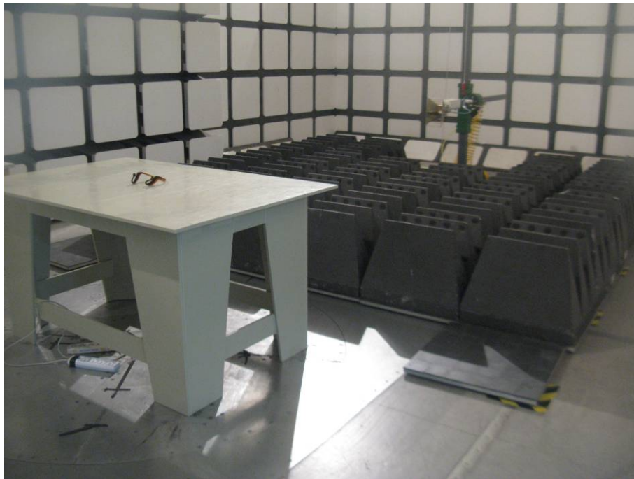
Above 1 GHz: Radiated Emissions - Front View (Transmitting mode)
