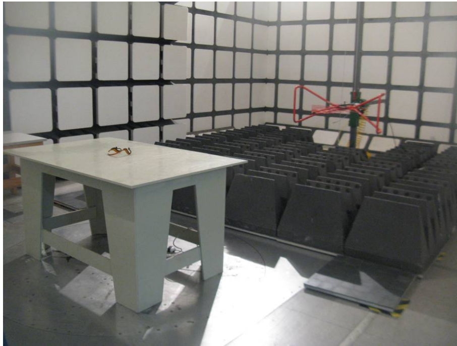
Below 1 GHz: Radiated Emissions - Front View (Transmitting mode)
