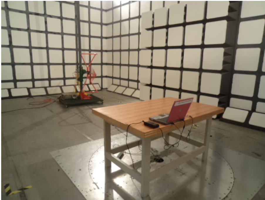
Radiated Emissions - Front View (Charging mode)
