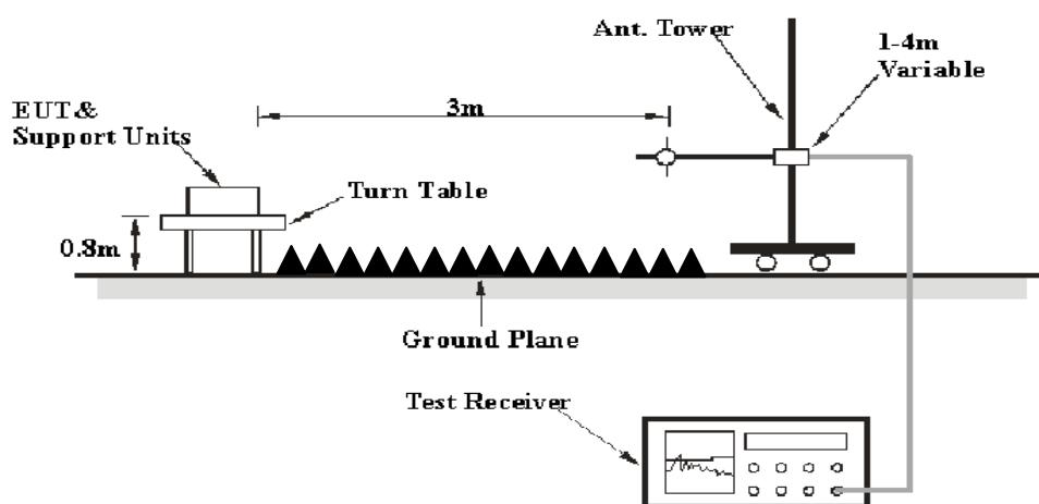
The radiated emission tests were performed in the 3 meters, using the setup accordance with the ANSI C63.4-2009. The specification used was the FCC 15.209 and FCC 15.247 limits.
