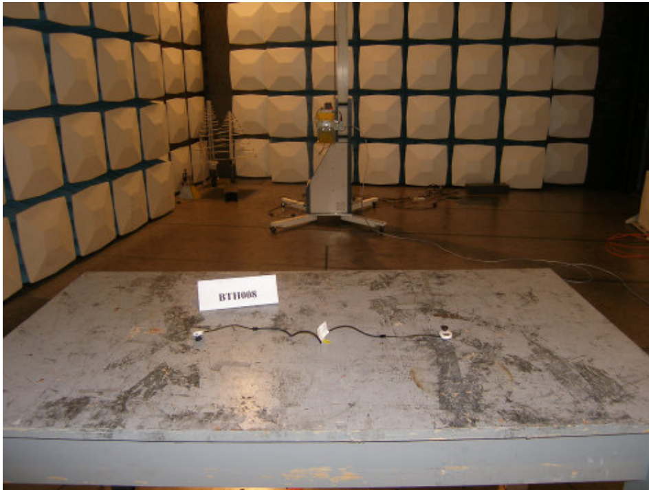
Photograph 3: Set-up for Radiation Measurement above 1GHz
