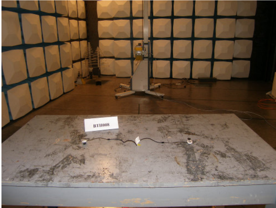
Photograph 3: Set-up for Radiation Measurement above 1GHz
