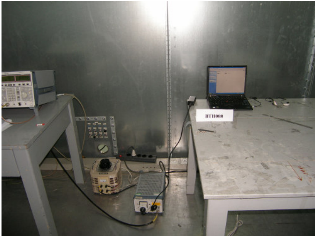
Photograph 1: Set-up for Conducted Emission
