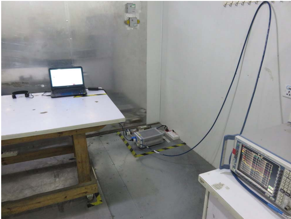
FCC RADIATED EMISSION TEST SETUP
