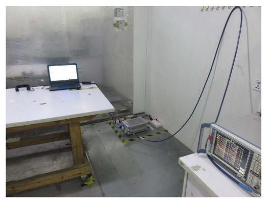
FCC RADIATED EMISSION TEST SETUP
