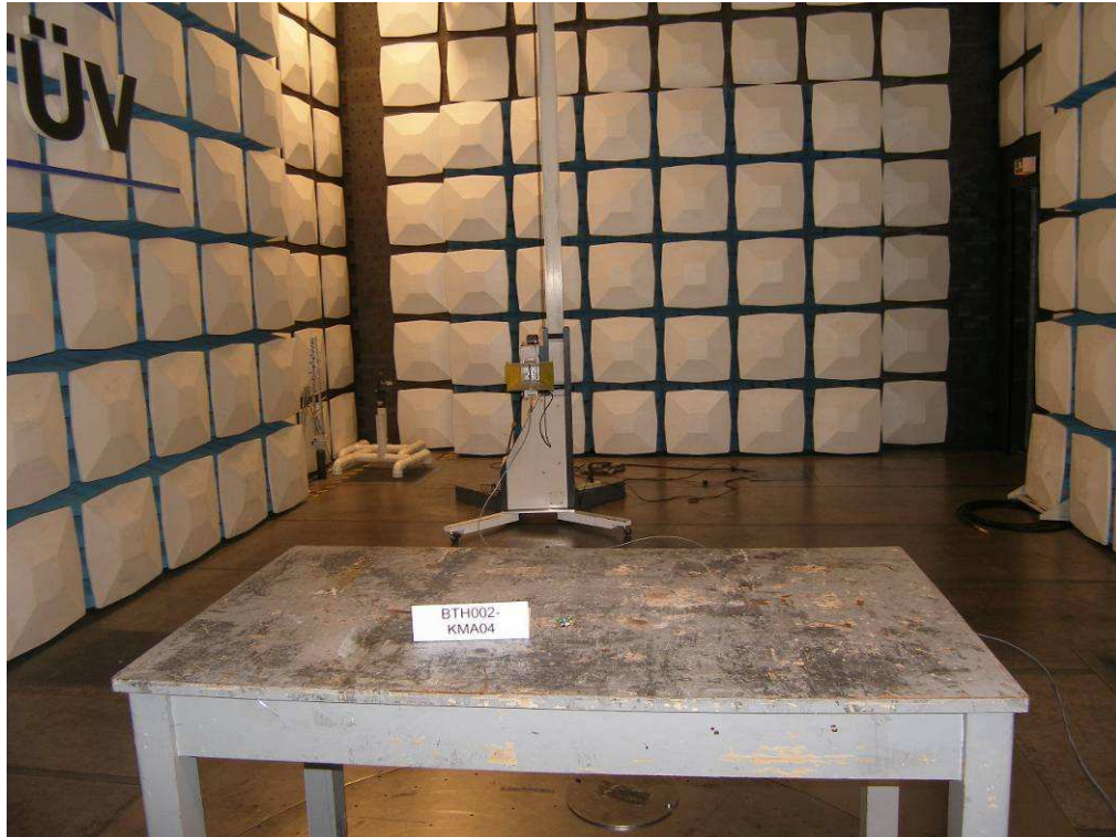
Photograph 4: Set-up for Spurious Emissions (18GHz-26GHz)
