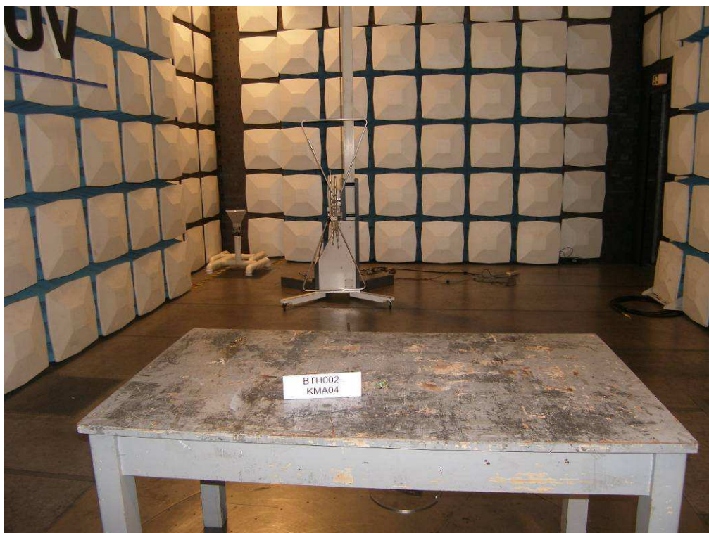
Photograph 2: Set-up for Spurious Emissions (30MHz-1GHz)
