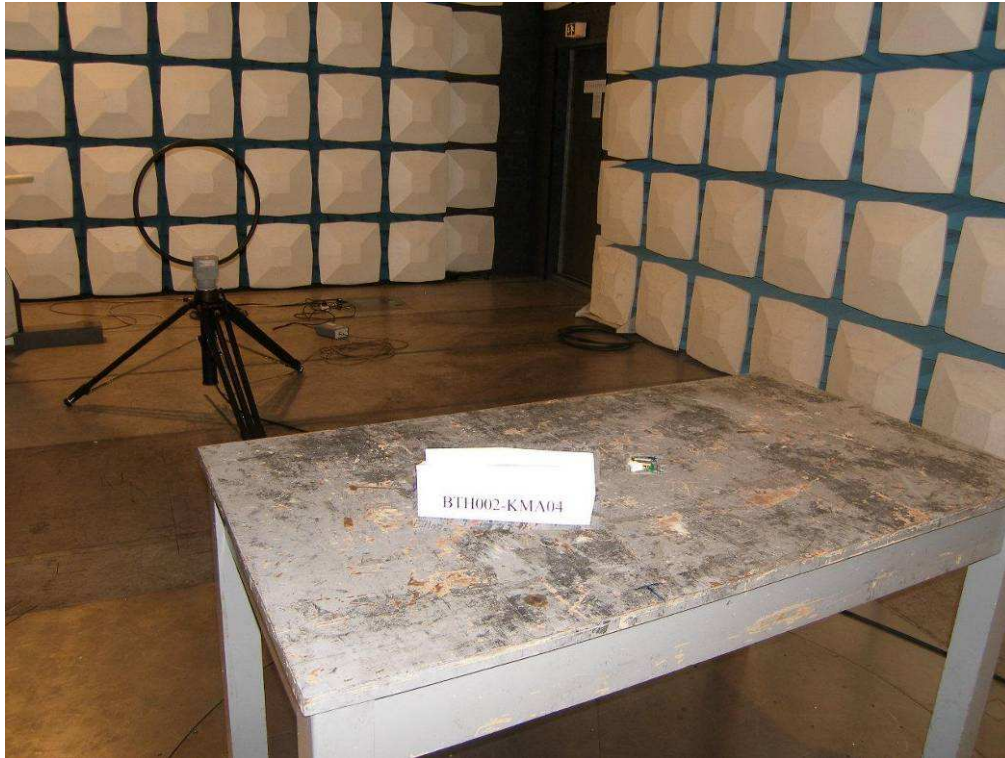
Photograph 2: Set-up for Spurious Emissions (30MHz-1GHz)
