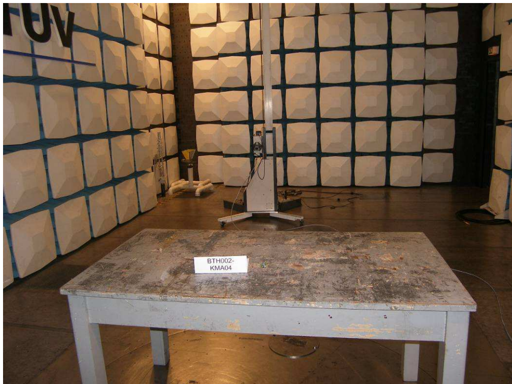
Photograph 4: Set-up for Spurious Emissions (18GHz-26GHz)
