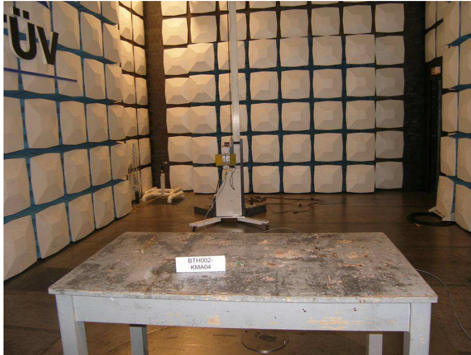
Photograph 4: Set-up for Spurious Emissions (18GHz-26GHz)
