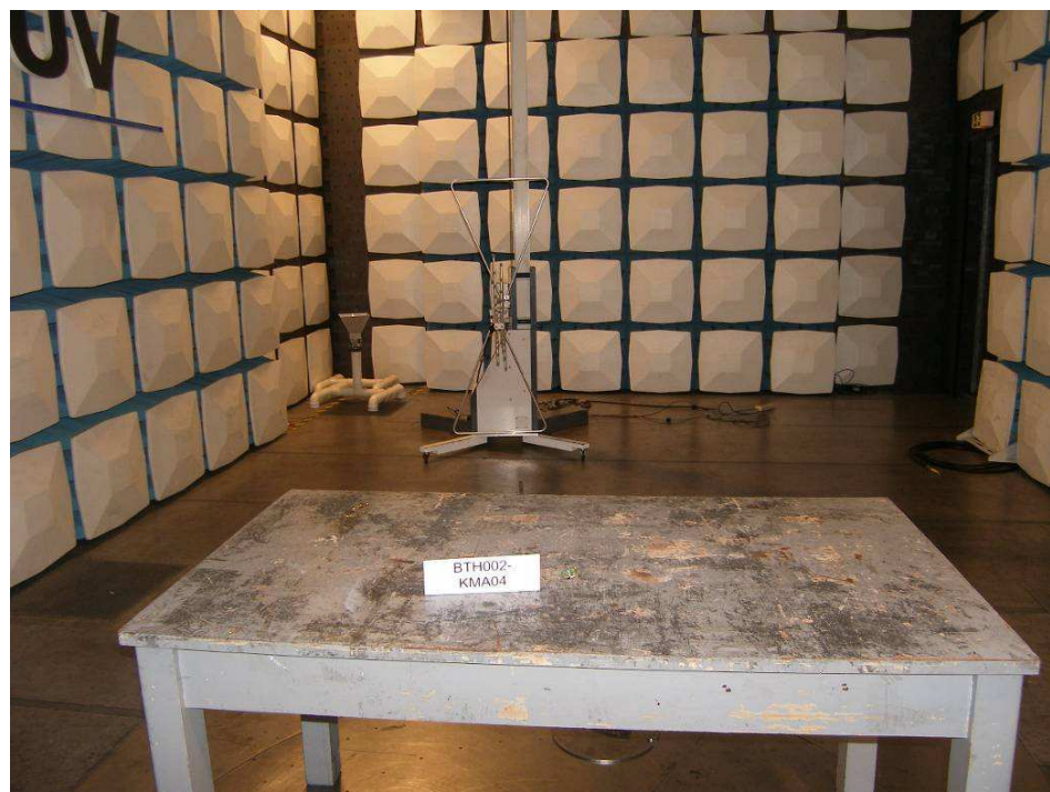
Photograph 2: Set-up for Spurious Emissions (30MHz-1GHz)
