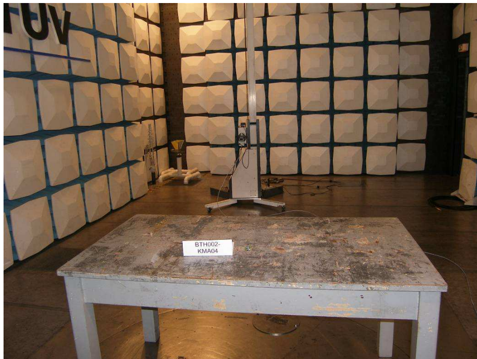
Photograph 4: Set-up for Spurious Emissions (18GHz-26GHz)
