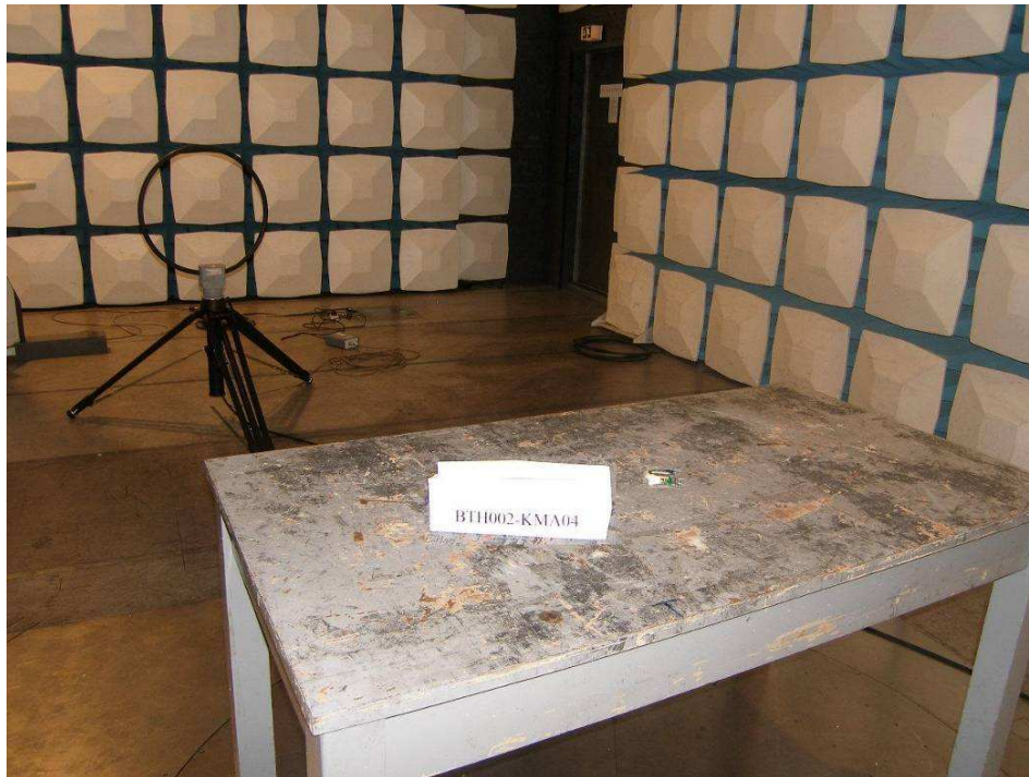
Photograph 2: Set-up for Spurious Emissions (30MHz-1GHz)
