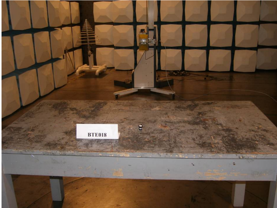
Photograph 2: Set-up for Radiation Measurement above 1GHz
