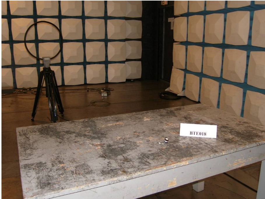
Photograph 1: Set-up for Radiation Measurement below 1GHz
