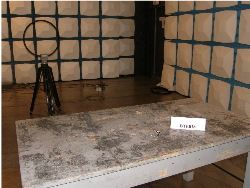
Photograph 1: Set-up for Radiation Measurement below 1GHz
