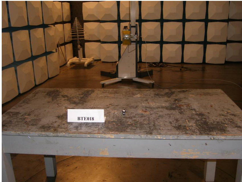
Photograph 2: Set-up for Radiation Measurement above 1GHz
