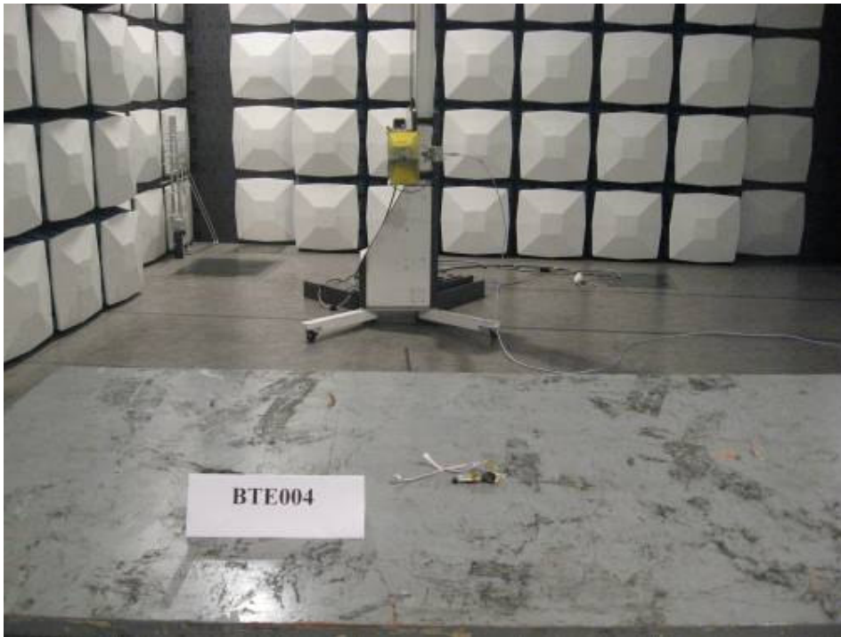
Photograph 2: Set-up for Radiation Measurement above 1GHz
