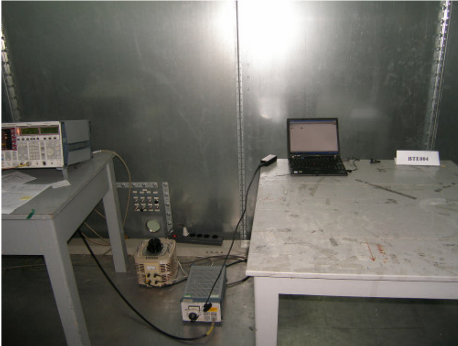
Photograph 3: Set-up for Conducted Emission
