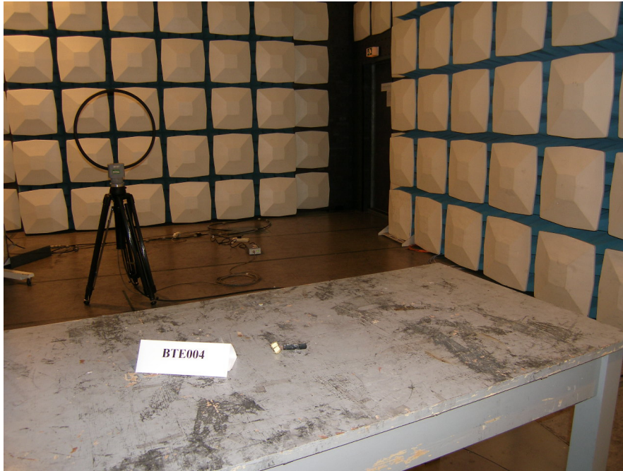
Photograph 1: Set-up for Radiation Measurement below 1GHz
