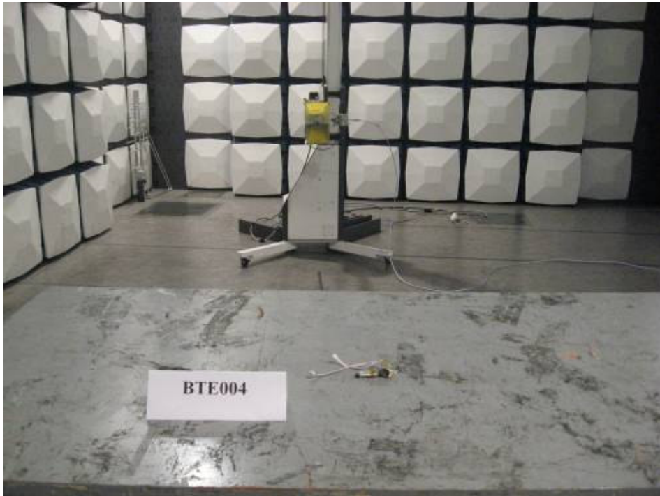
Photograph 2: Set-up for Radiation Measurement above 1GHz
