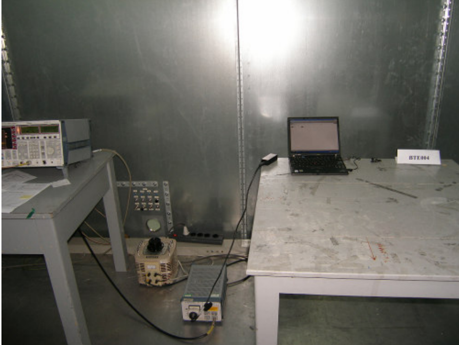
Photograph 3: Set-up for Conducted Emission
