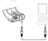
**8.** Charging for portable device This product has charge output jack (DC5V/1A). You can charge for portable device.
