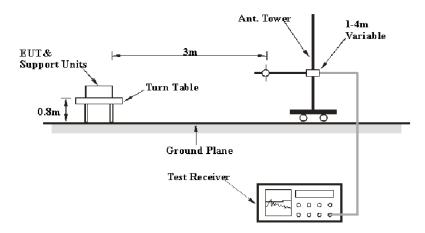
The radiated emission tests were performed in the 3 meters chamber B test site, using the setup accordance with the ANSI C63.4 - 2003. The specification used was the FCC Part 15.209 and FCC Part 15.239.
