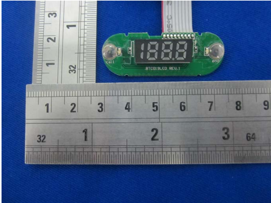
EUT – LED Board Top View
