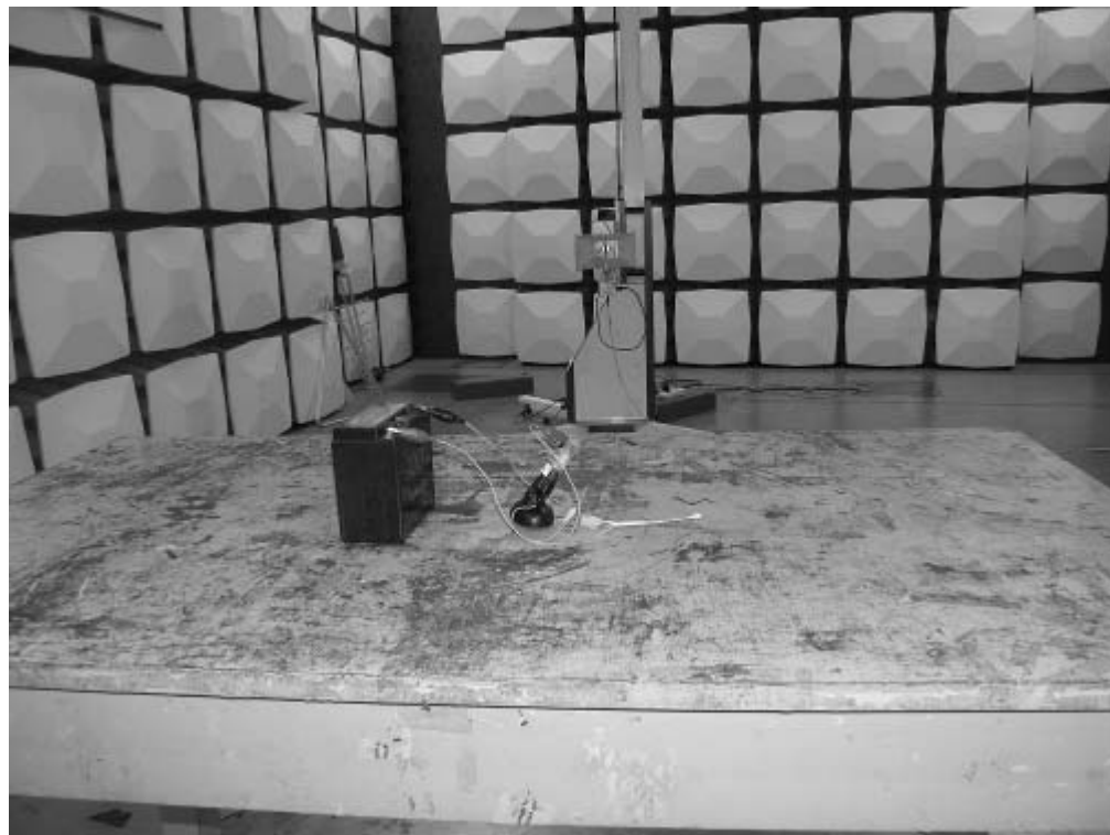
Photograph 2: Set-up for Radiation Measurement above 1GHz
