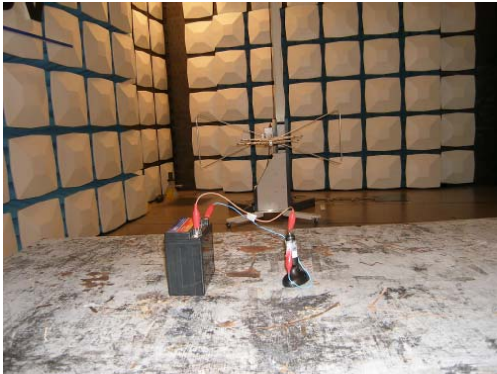
Photograph 1: Set-up for Radiation Measurement below 1GHz
