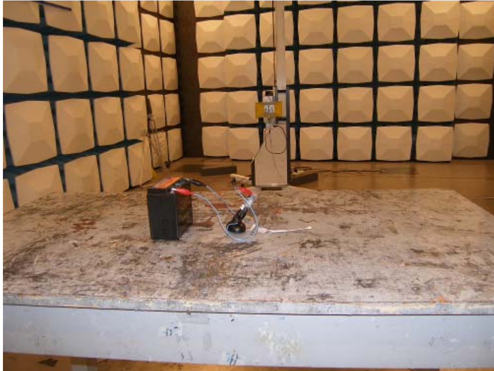
Photograph 2: Set-up for Radiation Measurement above 1GHz
