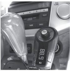
2) Rotating spin button of BTC008L to adjust its frequency to be the same as the car's FM radios. Frequency step is 0.2MHz. Clockwise rotating is increasing frequency, anticlockwise rotating is decreasing frequency.
