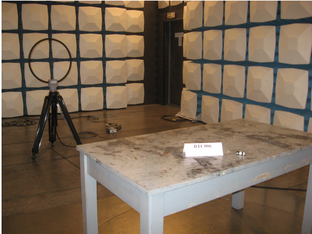
Photograph 1: Set-up for Radiation Measurement below 1GHz
