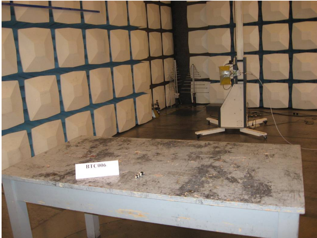
Photograph 2: Set-up for Radiation Measurement above 1GHz
