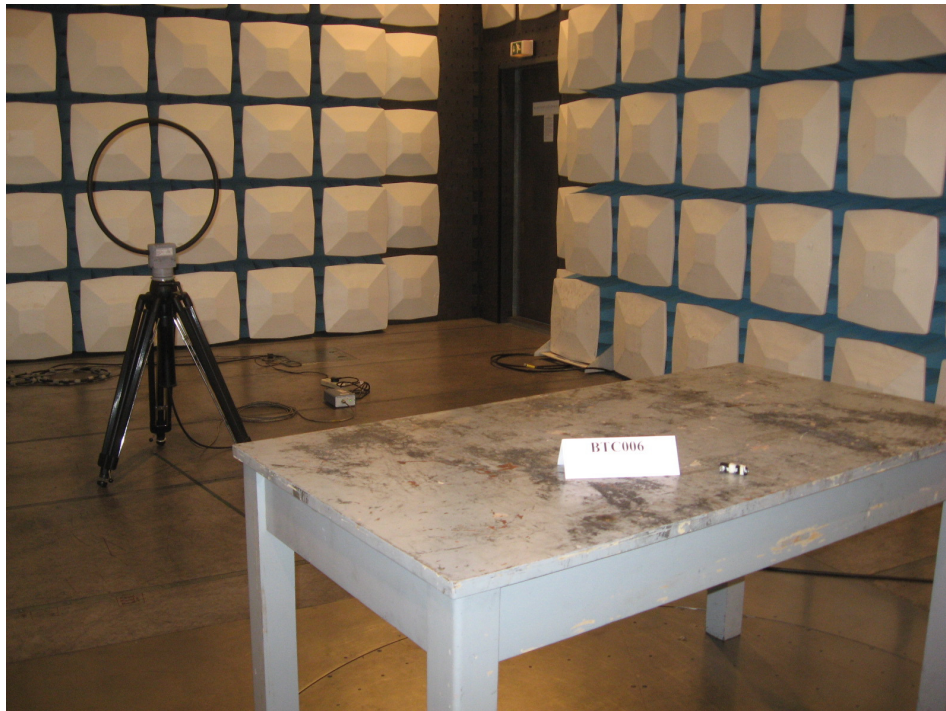
Photograph 1: Set-up for Radiation Measurement below 1GHz
