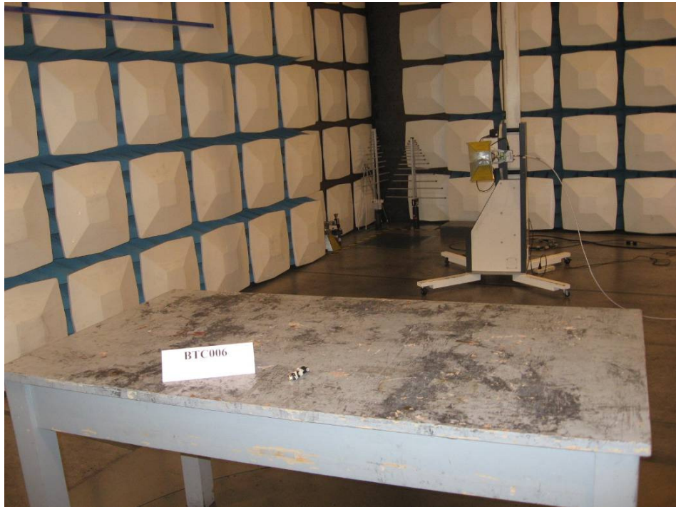
Photograph 2: Set-up for Radiation Measurement above 1GHz
